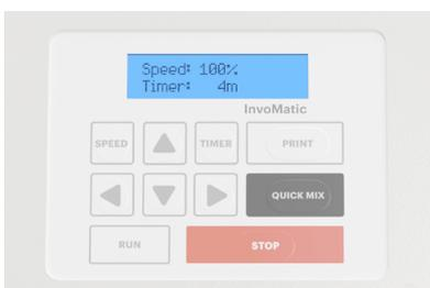
1. With the mixer in a stationary position, press the **"QUICK MIX"** button.
