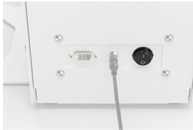
2. Turn the power switch located on the rear of the device to the "ON" position.
