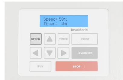
6. Once the desired speed is set, press the "SPEED" button again to set. This will stop the display flashing.
