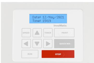
4. To store the date and time, press the **"STOP"** button and a buzzer will sound.
