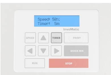
4. Once the desired time is set, press the "TIMER" button again to set. This will stop the display flashing.
