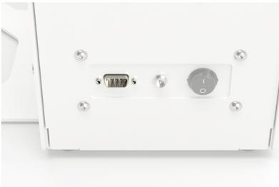
1. The **gako InvoMatic** is equipped with a Serial RS232 port, suitable for different models of thermal printers.
